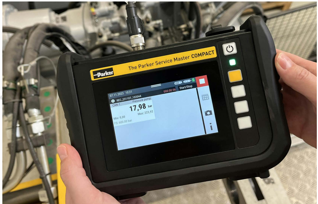
The SensoControl handheld device from Parker Hannifin's Quick Coupling Division can help diagnose maintenance issues with hydraulic systems in mobile and industrial applications.
