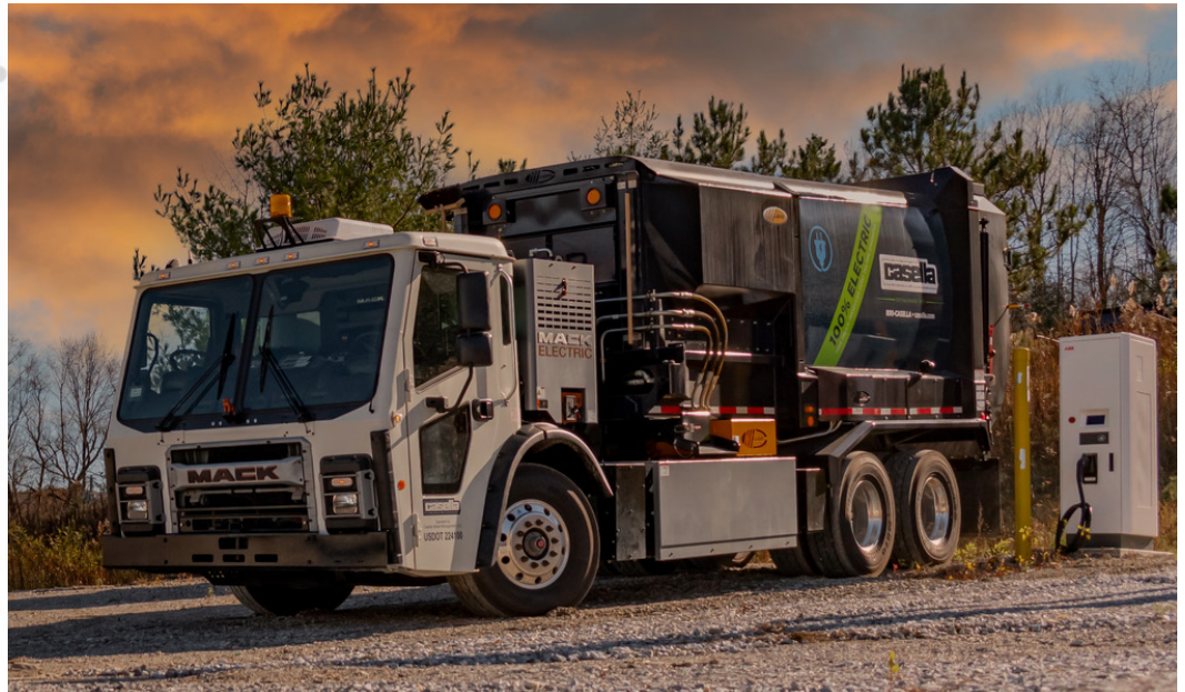
The latest version of the Mack LR Electric is powered by NMC lithium-ion batteries offering 42% more energy and 376 kWh total battery capacity. Mack Trucks
