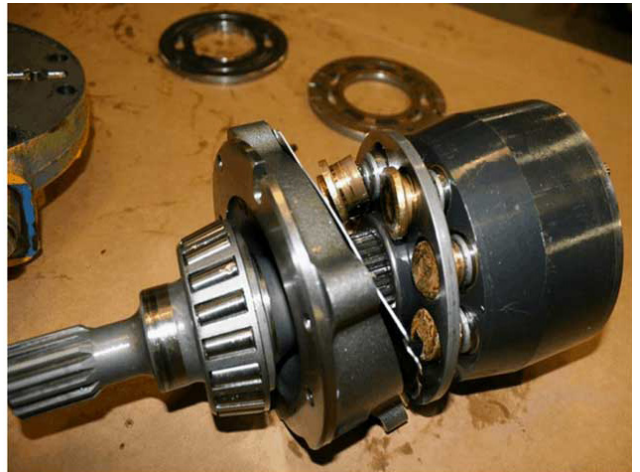
This pump motor was destroyed by contamination.
