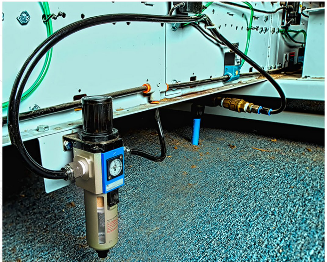
Air pressure regulators can be dedicated devices or combined with other functions like this Nitra filter/regulator combination from AutomationDirect, shown here installed on a conveyor.
