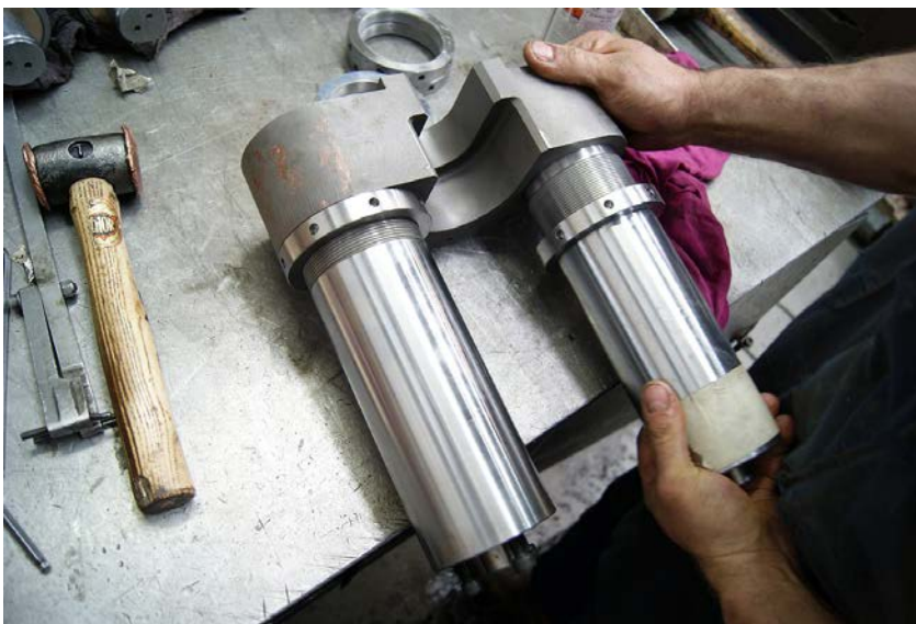
This highly specialized diver-operated subsea pin removal tool comprises two cylinders and two handles in one very small fabrication complete with camera mount.
