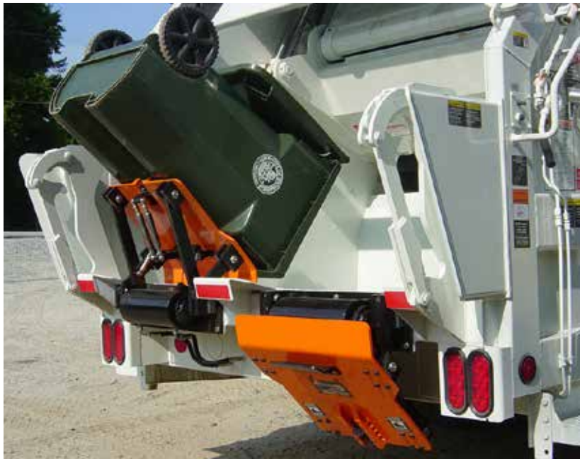
The helical rotary actuator (painted black) provides 220 deg. of rotation, completely emptying carts.
