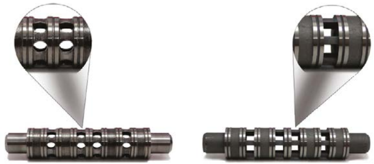
6. The original valve spool (left) had round holes, required with CNC machining. The spool redesigned for 3D printing has square holes with larger area to reduce pressure drop. (Courtesy of Aidro Srl)
