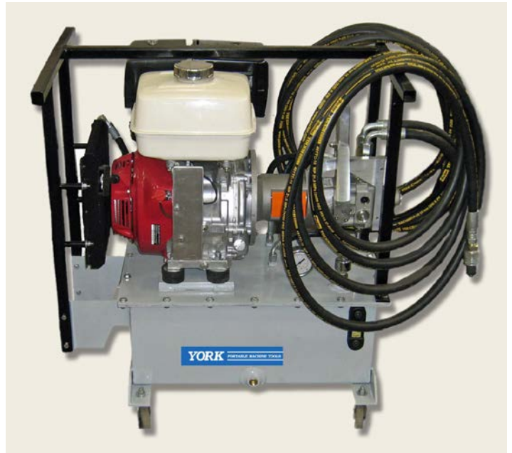
1. When a gasoline (shown here) or diesel engine will be the prime mover in driving a hydraulic power unit, sizing calculations will differ from those when using an electric motor. That's because electric motors develop very high starting torque, whereas gas and diesel engines develop roughly the same torque throughout their speed range. (Image courtesy of York Portable Machine, www.yorkmachine.com )
