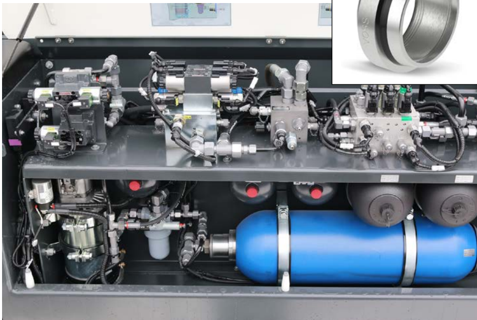
The hydraulic systems in Goldhofer's AST-2P/X aircraft tractor incorporate the soft-sealing ES-4 cutting ring from VOSS Fluid for long life without leakage.
