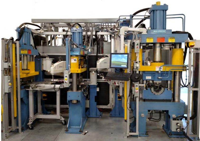
Here is the new Miba bearing manufacturing work cell. From left to right are the shearing press, the blanking press, and the forming press.
