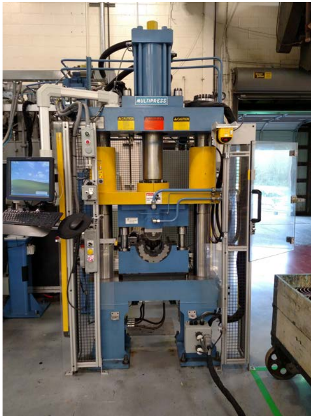
The preform cylinder is mounted in the blue tooling fixture below the yellow platen, which is moved by the main forming cylinder.
