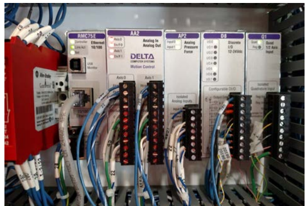
The RMC75E motion controller manufactured by Delta Computer Systems can control two motion axes and is available with a wide array of transducer and control interfaces.
