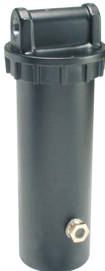
4. Point-of-use desiccant dryers are typically rated up to 60 scfm. This type of dryer can reach a pressure dew point down to -40°. The desiccant can also be regenerated (dried) while still in service.
