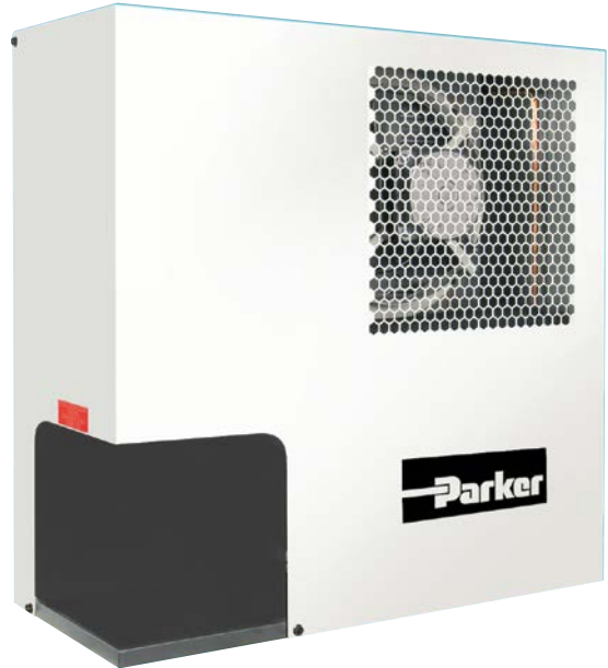
3. A refrigeration dryer removes water from a pneumatic system. This particular dryer accommodates flows from 10 to 175 scfm.
