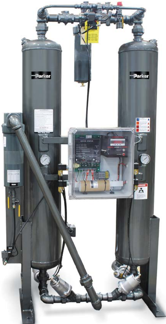
5. An example of a twin-tower regenerative desiccant dryer with flows from 25 to 800 scfm or more. This heatless dryer can reach pressure dew points down to -100° F.
