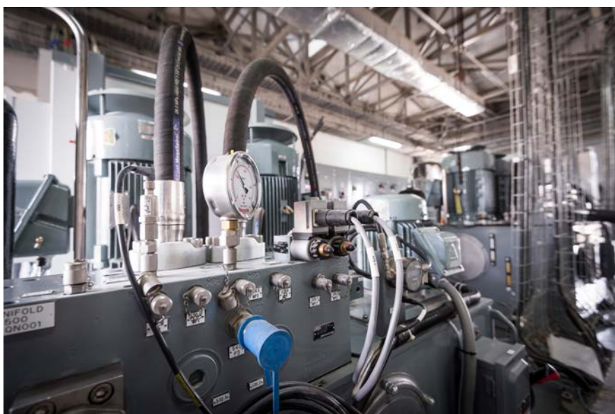
Here is a control block of a hydraulic power unit with pressure gauge.
