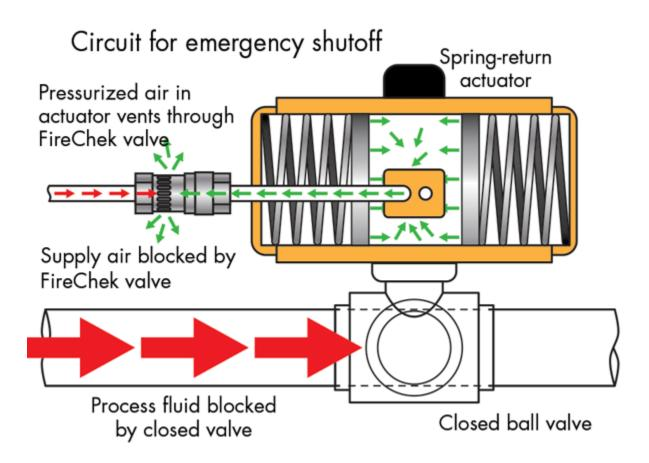
When the FireChek valve senses excessive heat from a nearby fire, it closes the air-supply line preventing the air from feeding the fire and simultaneously vents the spring-return actuator so it can return to its on, off, or throttling fail-safe position. The FireChek valve reacts within 25 sec. at a temperature rise rate of 30°F/min. and can exhaust 1-l of air in less than 1 sec. at 125 psi (8.62 bar).
